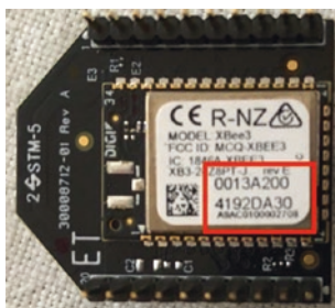
Figure 2-7. XBee address printed on the back of the module
